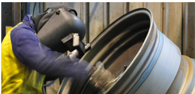
3. Welding (Section Replacement)
