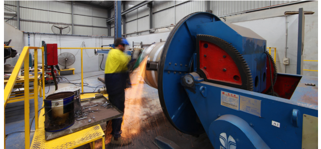
2. Back Grinding (Section Replacement)
