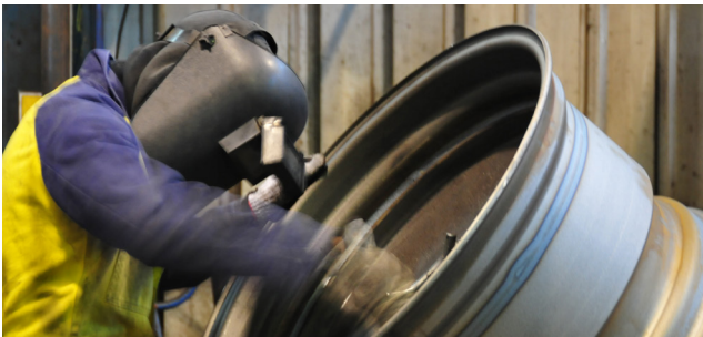
3. Welding (Section Replacement)
