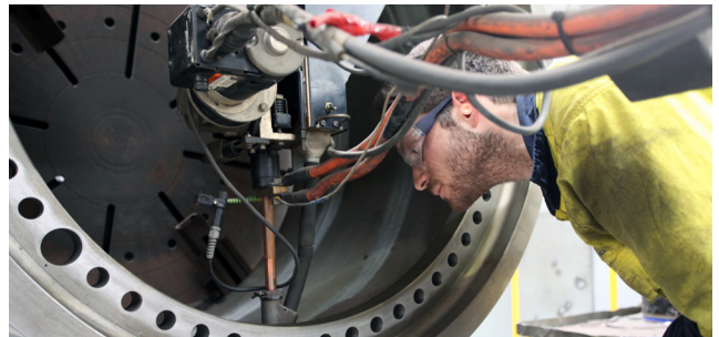
4. Welding (Section Replacement)
