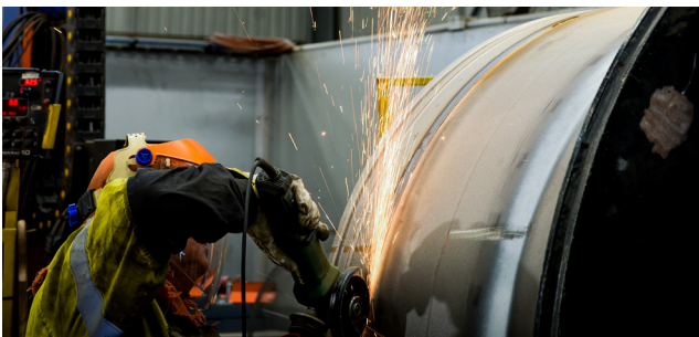
5. Machining (Repair Preparation)
