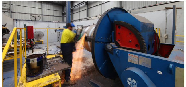
2. Back Grinding (Section Replacement)
