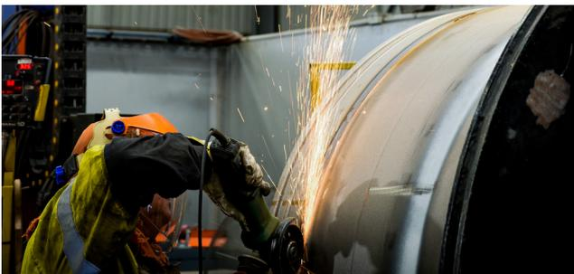
5. Machining (Repair Preparation)
