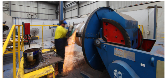
2. Back Grinding (Section Replacement)
